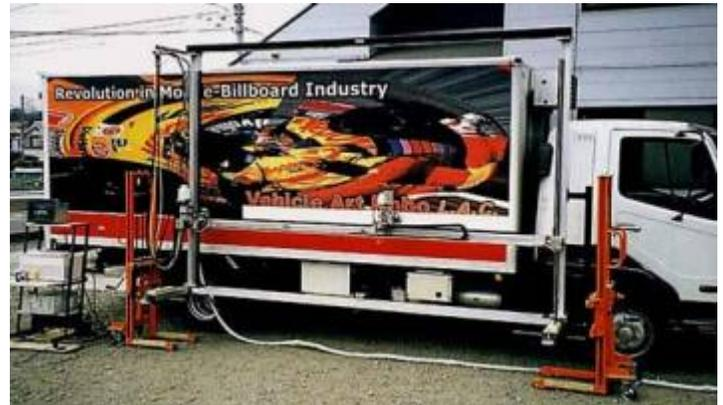
Printing of a 7m truck with a 4.5 machine
